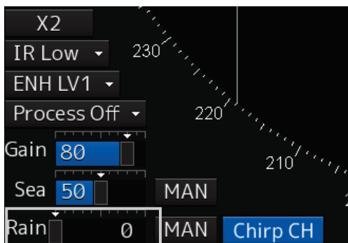
[Rain] (rain/snow clutter adjustment) slider
