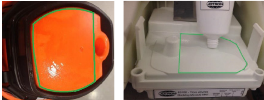
Applying of silicone grease
