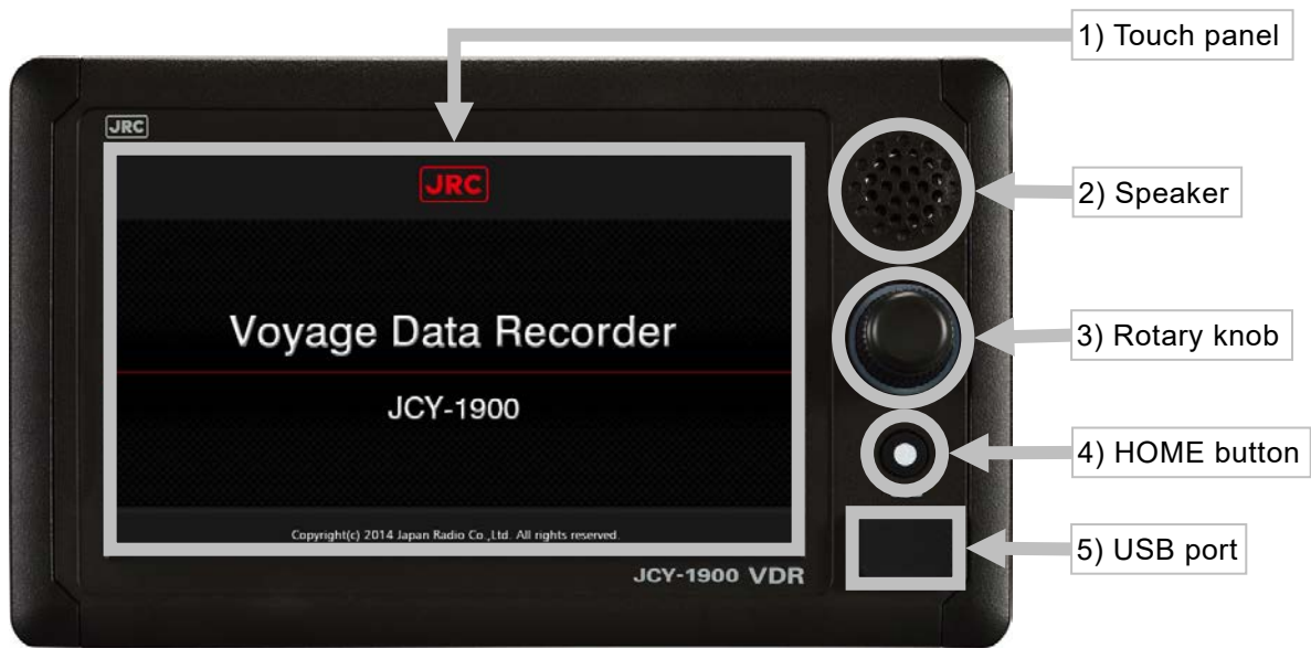
Figure 2-3 Name of each part of the Operation Panel Unit (OPU)
