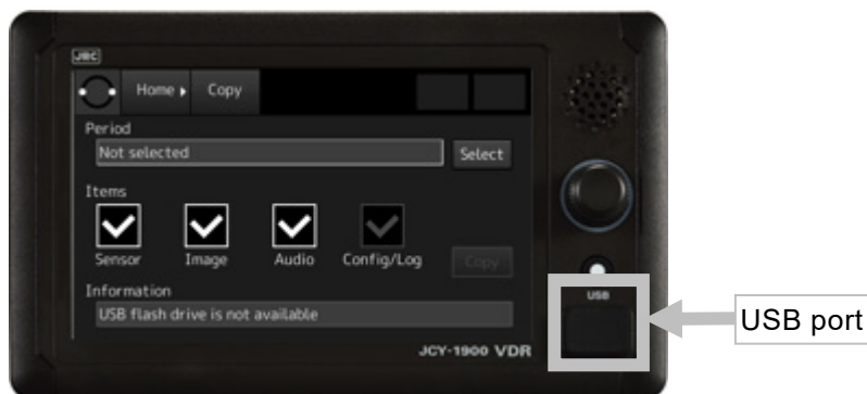
Figure 4-17 OPU's USB port
